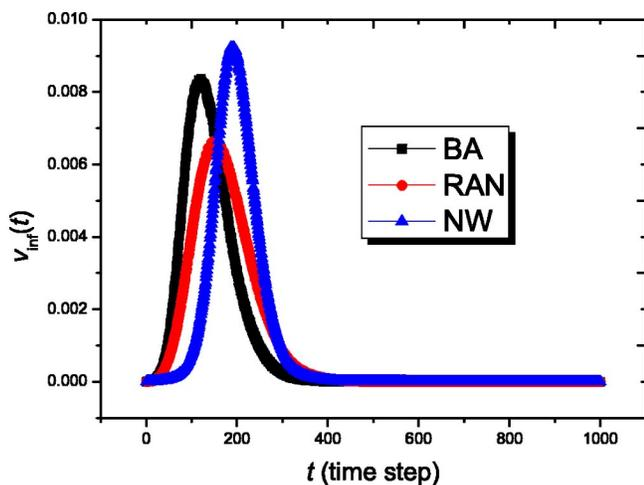
FIG. 10. (Color online) The spreading velocity versus time. The network order and spreading rate are the same with Fig. 9. The blue, red, and black curves (right to left) correspond to the cases of NW, RAN, and BA networks, respectively. The spreading velocity reaches a peak quickly. Before the peak time, the spreading velocities of the three kinds of networks satisfy the inequality  $v_{inf}^{BA} > v_{inf}^{RAN} > v_{inf}^{NW}$ . All the data are averaged over  $10^3$  independent runs.
