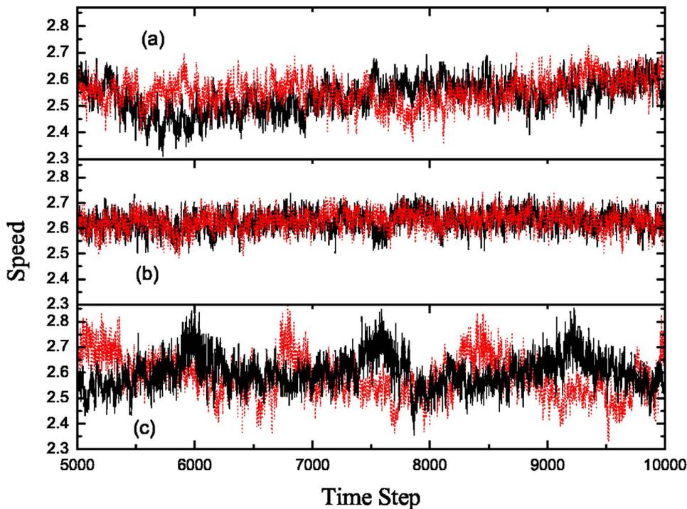
FIG. 5. (Color online) Average speed of each route by using (a) congestion coefficient feedback strategy, (b) mean velocity feedback strategy, and (c) travel time feedback strategy. The dark line and red dotted line represent route 1 and route 2, respectively. The parameters are set the same as in Fig. 2.
