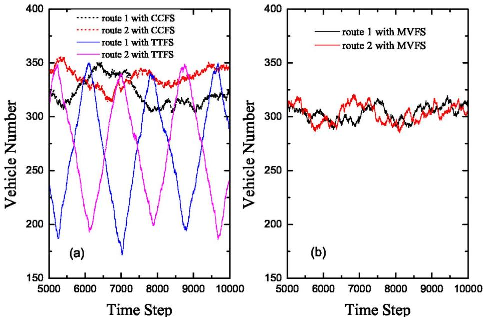
FIG. 3. (Color online) (a) Vehicle number of each route with travel time and congestion coefficient feedback strategies. (b) Vehicle number of each route with mean velocity feedback strategy. The parameters are set the same as in Fig. 2.
