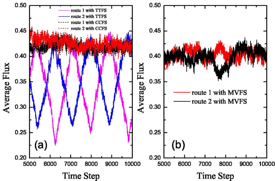
FIG. 2. (Color online) (a) Flux of each route with travel time and congestion coefficient feedback strategies. (b) Flux of each route with mean velocity feedback strategy. The parameters are  $L=2000$ ,  $p=0.25$ , and  $s_{dyn}=0.5$ .
