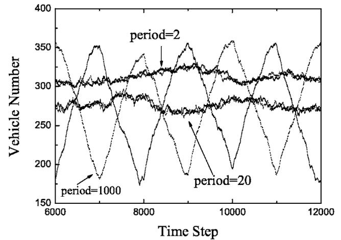
FIG. 9. Vehicle number of two routes as a function of time step by adopting CCFS for a different information feedback period. The parameters are the same as Fig. 8.
