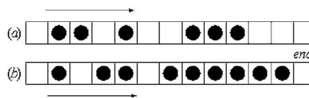
FIG. 1. Illustration of two routes with different congestion coefficient  $C$ . Each route has three clusters. According to Eq. (2),  $C_a=14$ ,  $C_b=41$ . Apparently, condition of route  $a$  is better than that of route  $b$ , which can be accurately reflected by  $C$ .
