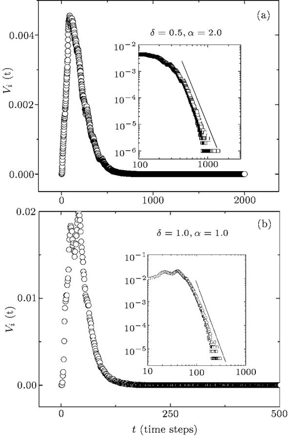
**Fig. 4.** Consider the cases of  $\delta < 1.0$  and  $\delta = 1.0$ . Here (a) and (b) show the spreading velocity at each time  $t$  in a BBV network with  $N = 10^4$ ,  $\omega_0 = 1.0$  and  $m = 3$ , when  $\delta = 0.5$ ,  $\alpha = 2.0$  and  $\delta = 1.0$ ,  $\alpha = 1.0$ , respectively. The inset shows the curves in a log-log plot. The data are averaged over 200 experiments.
