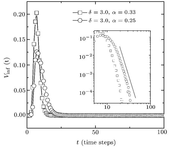
**Fig. 3.** Spreading velocity at each time  $t$  in a BBV network with  $N = 10^4$ ,  $\delta = 3.0$ ,  $\omega_0 = 1.0$  and  $m = 3$ , when  $\alpha = 0.33$  (square) and  $\alpha = 0.25$  (circle). The inset shows the curves in a log-log plot. The data are averaged over 200 experiments.
