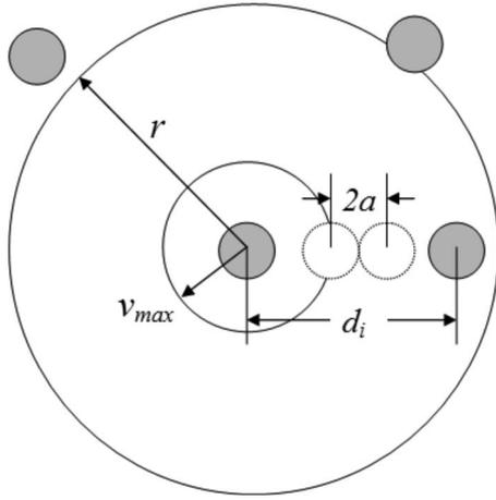
FIG. 1. Illustration of the current model with adaptive speed, where  $r$  denotes the horizon radius of an agent,  $d_i$  denotes the distance of the  $i$ th agent and its nearest neighbor,  $v_{\max}$  denotes the possibly maximal velocity, and  $a$  denotes the size of an agent. Accordingly,  $2a$  corresponds to the least distance of two agents.
