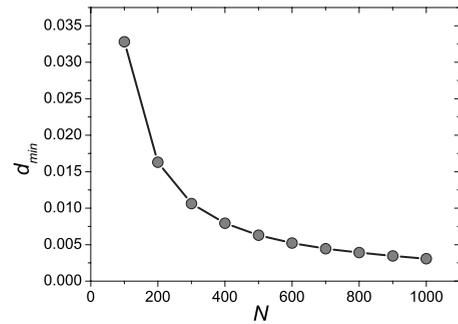
FIG. 6. Minimal geographical distance between pairs of agent in the stable state of the standard Vicsek model,  $d_{\min}$ , versus the number of agents,  $N$ . Each data point is the average of 1000 independent runs. The restriction to avoid collisions with agent size  $a=0.01$  corresponds to  $d_{\min} > 0.02$ .
