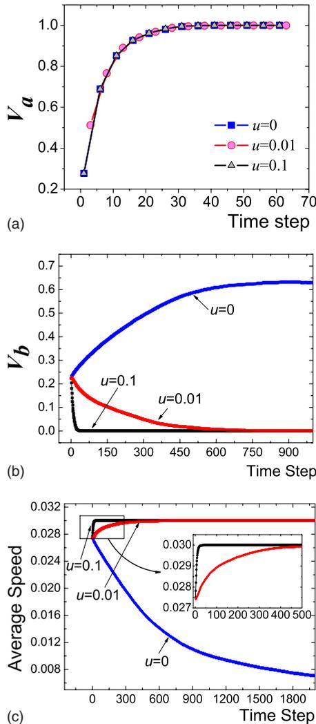
FIG. 5. (Color online)  $V_a$ ,  $V_b$ , and the average speed versus time steps under different repulsion strengths. The parameters are set as  $L=5$ ,  $N=300$ ,  $r=1$ ,  $v_{\max}=0.03$ , and  $a=0.01$ . All the data come from the average results of 500 independent runs.
